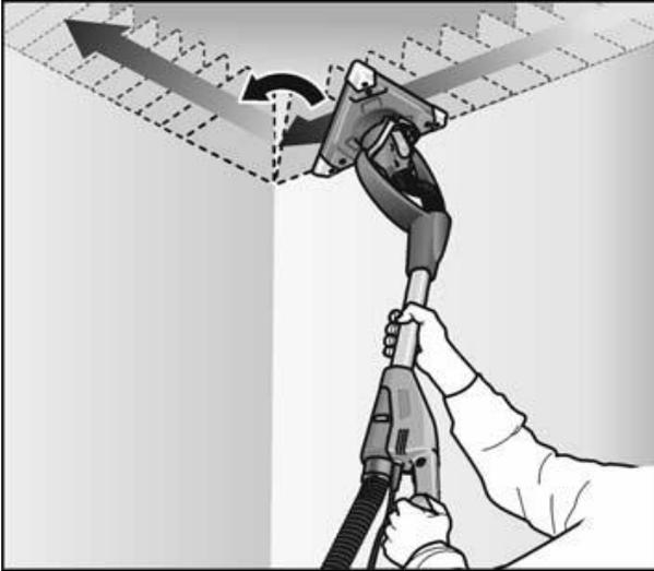
As the triangular sanding head can revolve on bearings, it can sand right into the corners of the wall/ceiling.
